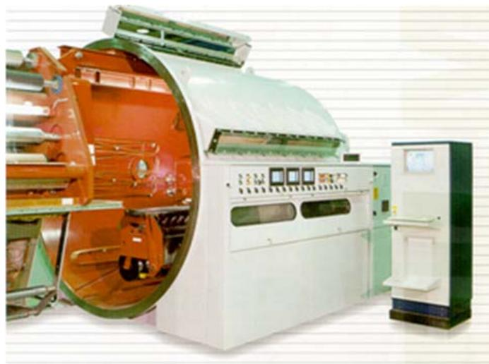
Fig. 7: Metallization chamber.
